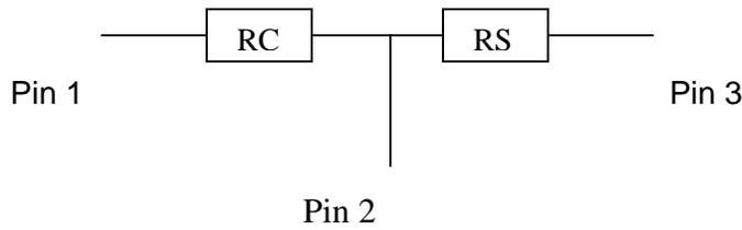
**Figure 3. KHS-200 MEMS Micropellistor Circuit Diagram**
