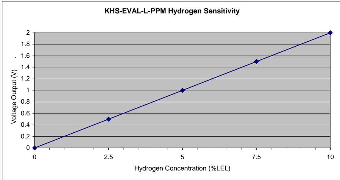
Figure 5. KHS-EVAL-L-PPM Output Voltage from 0 to 10% LEL
