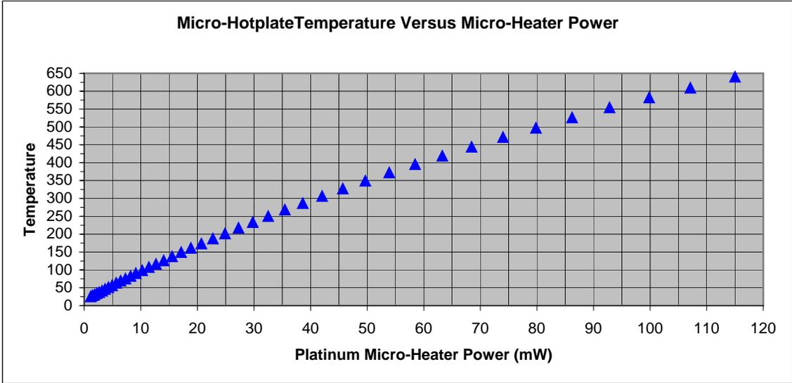
Figure 4. Temperature Versus Micro-Heater Power (mW)
