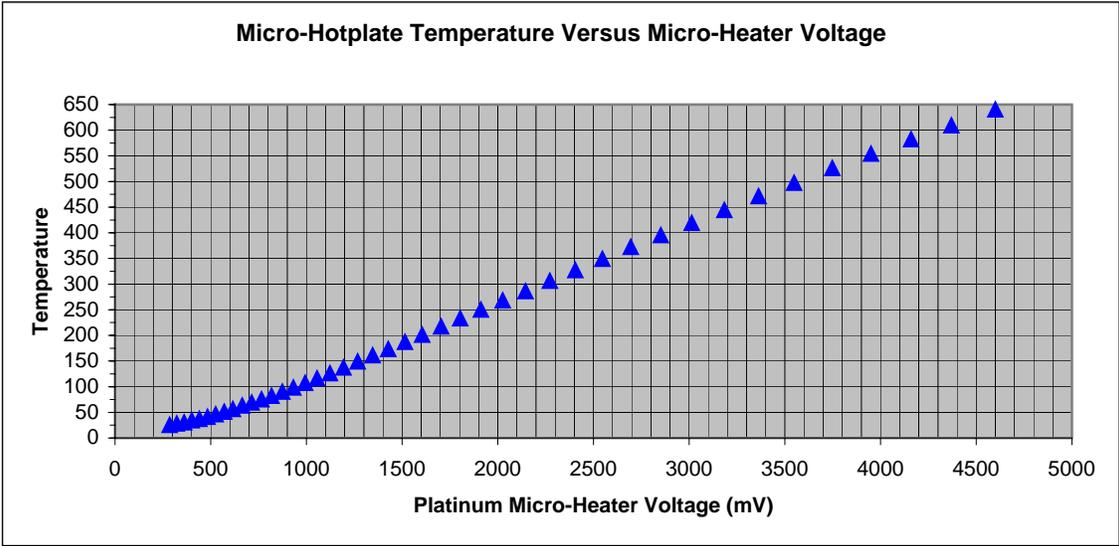
Figure 3. Temperature Versus Micro-Heater Voltage (mV)
