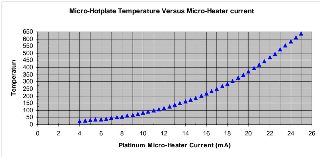
Figure 2. Temperature Versus Micro-Heater Current (mA)
