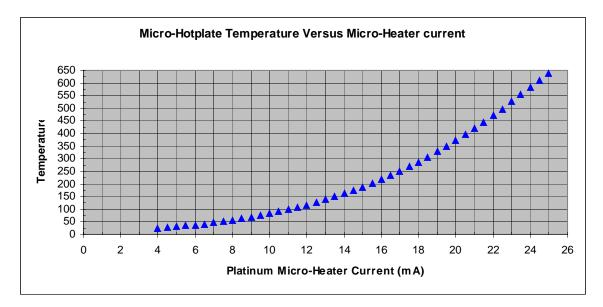
Figure 2. Temperature Versus Micro-Heater Current (mA)
