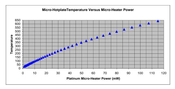
Figure 4. Temperature Versus Micro-Heater Power (mW)
