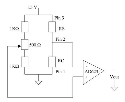
Figure 4. KHS-200 MEMS Micropellistor Operating Circuit
