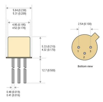
Figure 2. KHS-200 MEMS Micropellistor 3-Pin TO-18 Package
