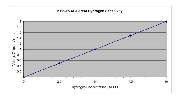
Figure 5. KHS-EVAL-L-PPM Output Voltage from 0 to 10% LEL
